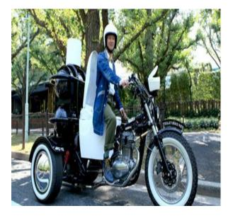
b) Biogas motorcycle in Japan (Source: http://buffetoblog.wordpress.com /2011/11/09/a-motorcycle-fueled-by-poop/)
