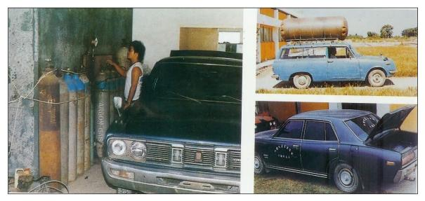
Figure 11: Biogas bottling and utilisation in vehicles in Taiwan (Source: Su J.J., 2011)
