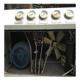
Figure 21. Newly procured high pressure small-scale compressor at IIT Delhi (Source: Authors)
