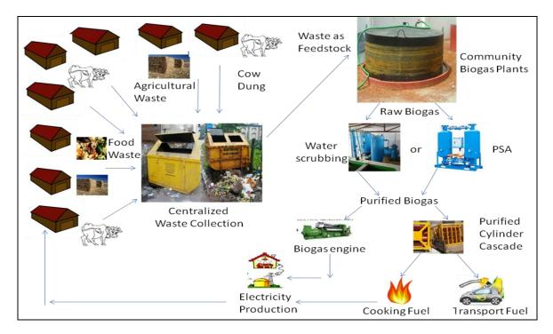
Figure 32. Schematic diagram of Biogas Entrepreneurship Model I (Source: Author).
