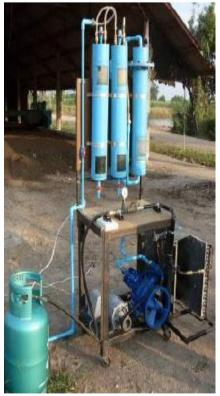
d) Biogas purification system
