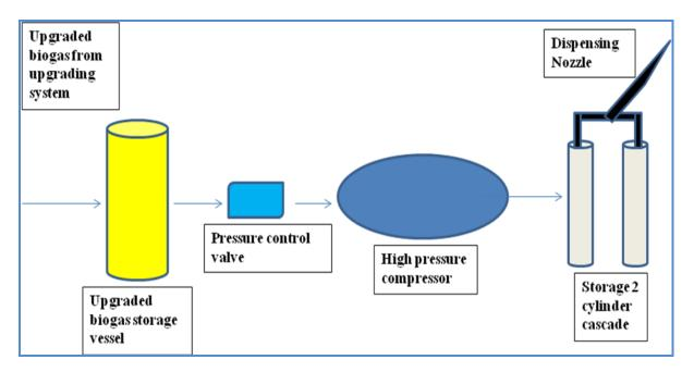
Figure 16. Upgraded biogas bottling system (Source: Authors)
