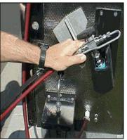
b) CNG nozzle and dispenser (Source: http://daq.state.nc.us/motor/cn g/crownvic.shtml)
