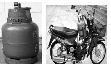
b) LPG cylinder c) Motor-cycle run on LPG
