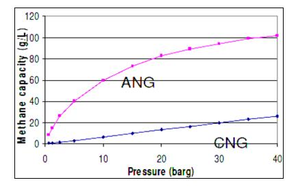
**Figure 27.** Methane storage capacity in CNG and ANG cylinders (*Source: Judd R. et al, ANG Technology, Germanishar Lloyd, http://www.apinvest.co.in/inside/pdf\_gas\_glis.pdf*)
