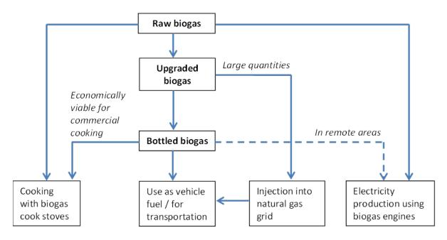
Figure 1. Different uses of biogas (*Source: Authors*)
