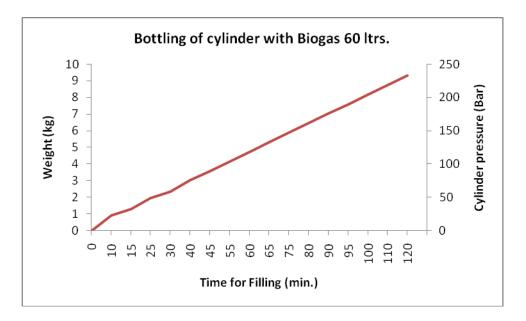
Figure 26. Graph showing the amount of upgraded biogas filled in 60-litre CNG cylinder (*Source: Authors*)
