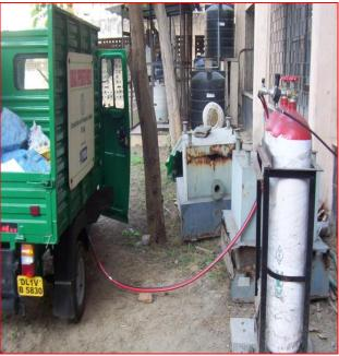
Upgraded biogas being dispensed into biogas vehicle
